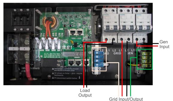
Figure 14.0 - AC Power Input/Output Wiring Connection Points
