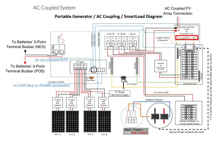
Figure 13.0 – AC Coupled AccESS Sol-Ark Wiring Diagram
