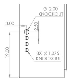
Figure 5.0 – AccESS Cabinet Knockouts (sides)
