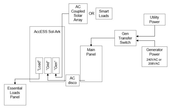
Figure 15.0 - Generator Wiring in Grid-Connected AC Coupled Systems
