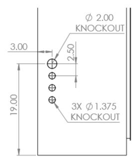
Figure 16.0 - AccESS Cabinet Knockouts (Sides)
