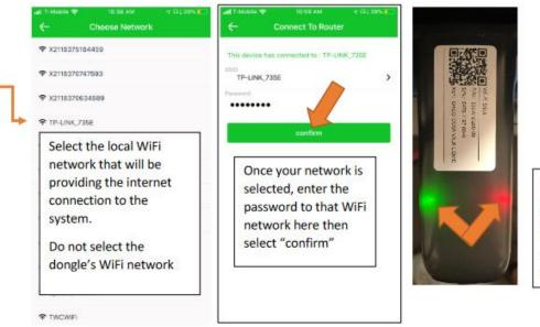
If successful, the dongle will have one red and one green light. It takes about 60sec for the lights to turn on after setup.
