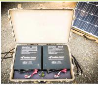
Two OES3.4 Smart-Tech batteries provide 7 kWh of storage at onethird the weight, and less than half the space of the original lead acid batteries deployed by the U.S. Army and Marine Corps.
