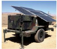
The OES 3.4 batteries store up to five times as much power from mobile PV panels as the toxic lead acid batteries they replaced.
